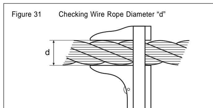
**WARNING: REPLACEMENT WIRE ROPE MUST BE SAME SIZE, GRADE, AND CONSTRUCTION AS THE WIRE ROPE SPECIFIED BY THE SUPPLIER! (See pages 7, 11)**
