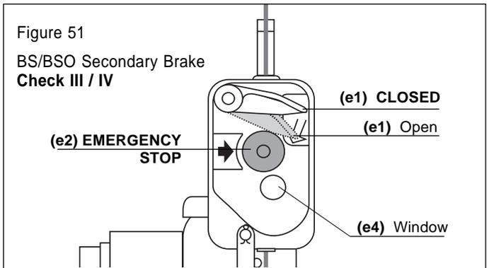
d) Check EMERGENCY STOP button and push-button control according to page 12.
