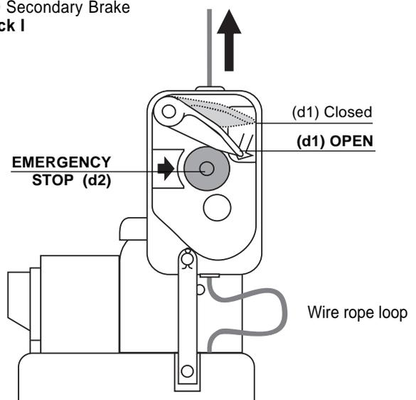
II Lift platform 3 ft. (1 m) above ground or safe surface, and push EMERGENCY STOP button (d2) of the BSO secondary brake (Fig. 29). Lower the platform to check that the BSO secondary brake holds the load. Raise platform until the hoist supports the load. Reset (d1) to the open position.
