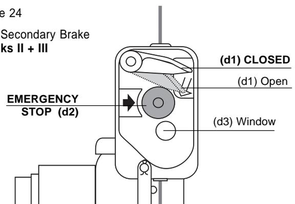
Raise platform until the hoist supports the load. Reset (d1) to the open position.
