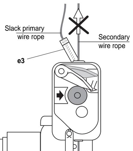
tilts to the side to close BS/BSO secondary brake for the secondary wire rope (Fig. 49).
