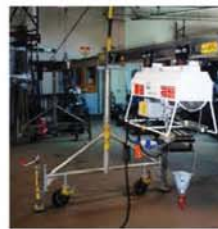
Beta Max Gemini Plus 110v 6000lb/72000lb Hoist on a rolling roof rig enable you to have an 14' cantilever.
